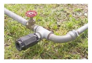
8. Main Pump Body at End of Type B Drive Pipe
